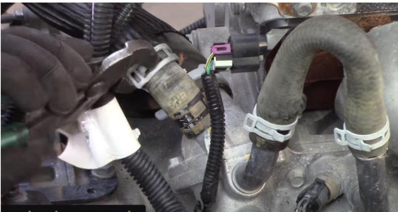
Use a 15mm wrench to disconnect and remove the powertrain ground
