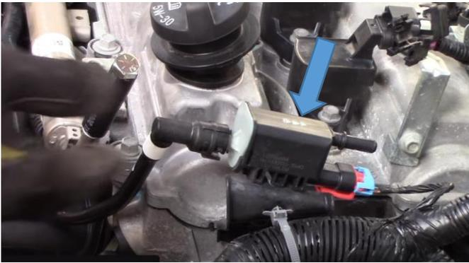
Use a 10mm socket to remove the evap valve
