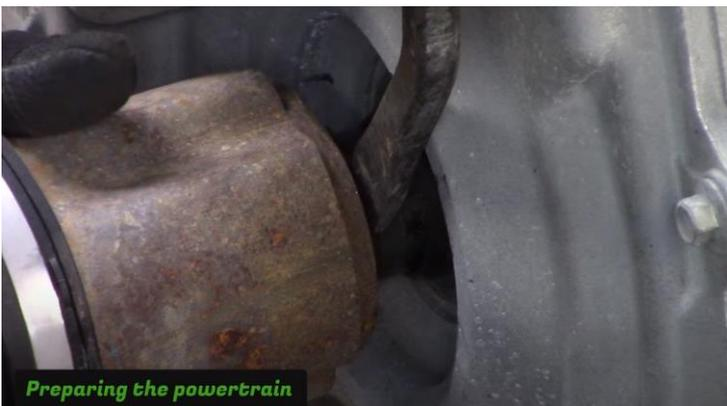
Spray the O2 sensor with penetrating oil
